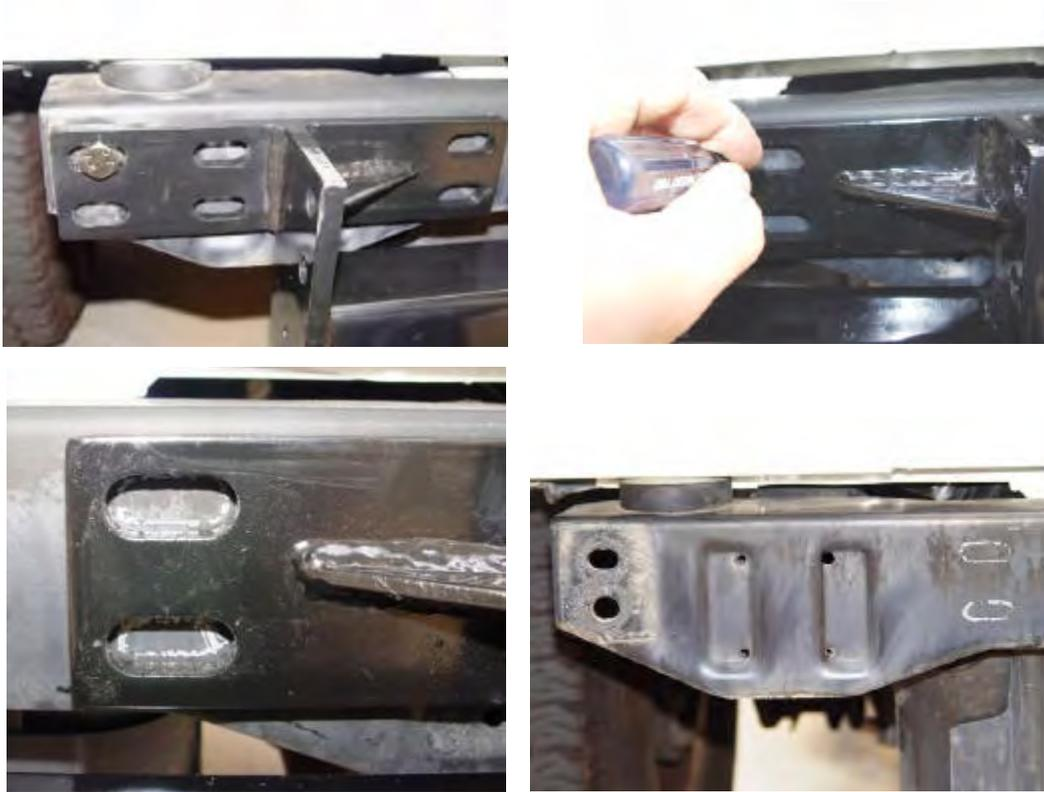
**Step (3)** Drill holes into rear cross member. **WARNING ... BE VERY CAREFUL WHEN DRILLING MOUNTING HOLES. THE FUEL TANK IS LOCATED JUST BEHIND THE CROSS MEMBER.** Great care will be needed to avoid puncturing the fuel tank. Use a small 3/16" drill bit for a starter hole. After small holes have been drilled, enlarge them with a 1/2" drill bit. **BE VERY CAREFUL TO AVOID HITTING THE FUEL TANK WHEN DRILLING.**
